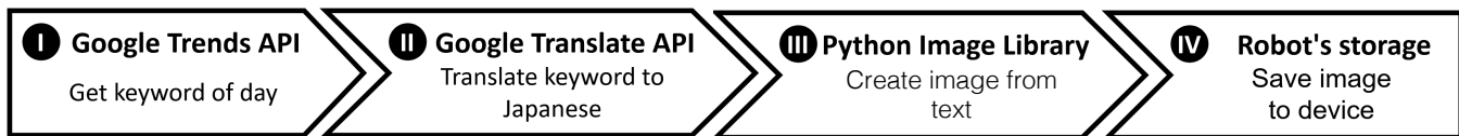
Fig. 2. Workflow for topic selection: Gaka-chu first (I) selects the English keyword with the largest number of searches that day in Google Trends, (II) translates the keyword into Japanese characters, (III) converts the resulting text into an image, and (IV) uses the image as an input for the physical painting process.
