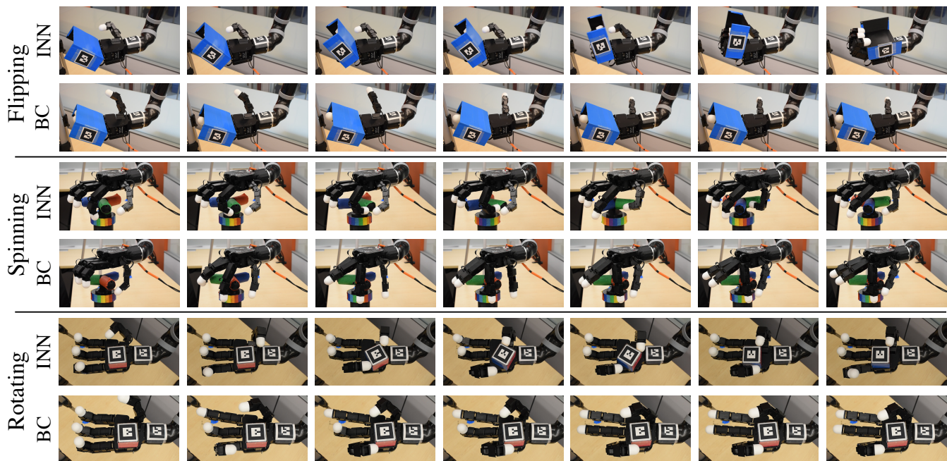
Fig. 3: Robot runs for both state-based (INN) and image-based (VINN) non-parametric nearest neighbors along with state-based parametric behavior cloning (BC) are visualized across the three tasks. INN performs the best across all three tasks, while VINN is able to solve the flipping and rotating tasks. BC is unable to solve any task and suffers from distributional mismatch [38].
