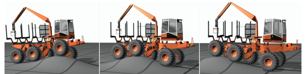
Fig. 5. Sequential snapshots of the vehicle traversing a 1 m tall gaussian bump, avoiding chassis roll and wheel slip.
