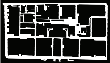
Fig. 3. The prior knowledge of Zhejiang Lab park represented as a grid map.
