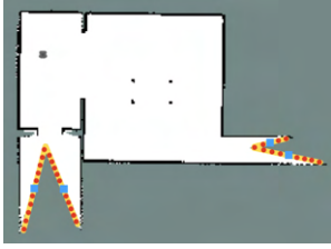
Fig. 4. Detect and Cluster frontiers, frontiers(red), clustered frontiers(yellow), and center point of clustered frontiers(blue)
