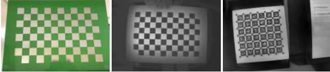
(a) RGB image of PCB checkerboard. (b) Thermal image of heated PCB. (c) Image of AprilTag recovered from events.
