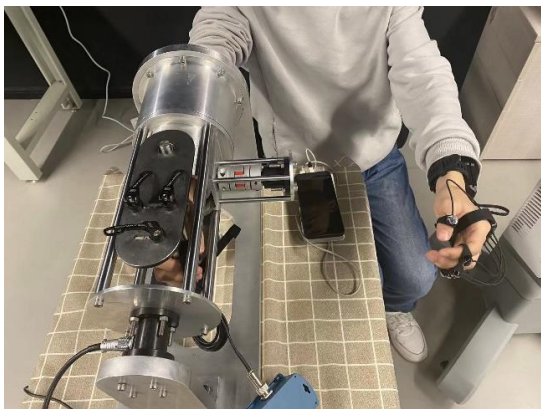
Fig. 3. Experimental set-up for the mirror bilateral training. The left hand wore the data glove and the right hand attached DTS sensor
