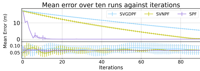
Fig. 2: Mean error of gradient-based methods against number of iterations for the first time step (top) and 15 th time step (when all methods have converged to the true state) (bottom). SPF converges earlier to the correct state while other methods take much longer. Bottom subplot shows the performance in tracking mode indicating instant convergence requiring a few iterations.
