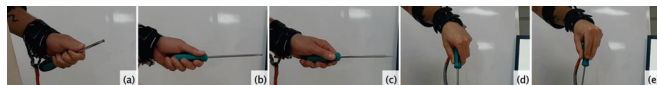
Fig. 8. Grasps of a screwdriver by subject 9. The classification model certainties p(\text{screwdriver}) about the object are (a) 94.92%, (b) 93.05%, (c) 90.66%, (d) 94.06% and (e) 93.78%.
