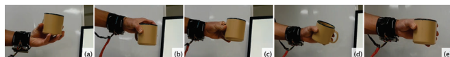
Fig. 7. Grasps of a drinking cup by subject 4. The classification model certainties p(\text{cup}) about the object are (a) 98.65%, (b) 95.71%, (c) 85.43%, (d) 96.77% and (e) 92.96%.
