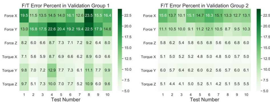
Fig. 8. Ten independent tests were performed on both validation group 1 and validation group 2 to verify the repeatability. The error percentage of each test is calculated using Eqn. 12. The values in the left figure reflect the overall error level (error caused by the DNN prediction deviation and uncontrollable errors), and the values in the right figure reflect the uncontrollable error level. The error level of validation group 1 is generally higher than that of validation group 2, the gap between 2 groups' accuracy reflect the error caused by the DNN prediction deviation. The results show this experiment has a good repeatability.
