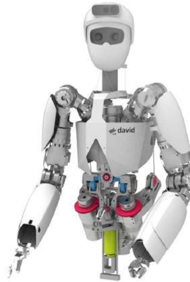
Fig. 1. CAD model of the upper body of the DLR David robot with the proposed torso joint
