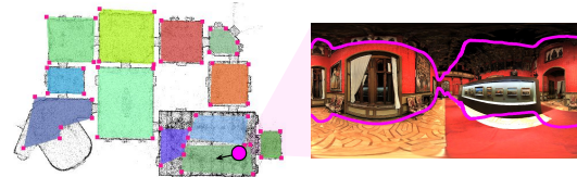
Fig. 7. Failure Case. We show that the noise from the 360-layout estimation could cause the room identification to fail, making a large room split into small parts. Note that the floor is occluded by a large furniture.
