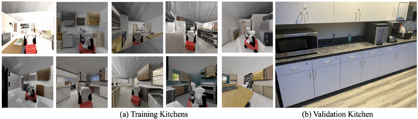
Fig. 3: Train and Validation Environments. Fig. (a) exhibits a subset of simulated kitchen environments in which the TIAGo robot learns each mobile manipulation primitive skill. The TIAGo robot is equipped with two Robotiq parallel-jaw grippers and five cameras capturing five images at 3Hz. To narrow the domain gap, we use a real world kitchen for validation (Fig. (b)), and then evaluate M-EMBER on three kitchens.
