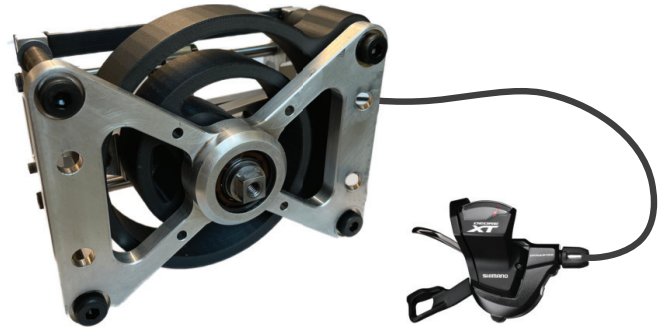
Fig. 1. Variable stiffness spring with human-selectable stiffness.
