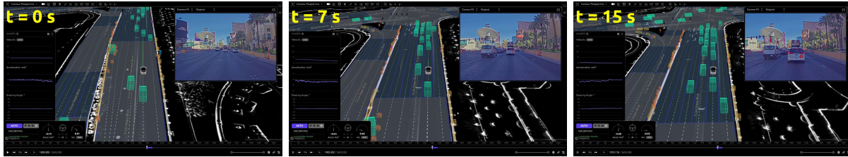
Fig. 5. Smoothly stopping behind a vehicle in dense traffic on the Las Vegas Strip.
