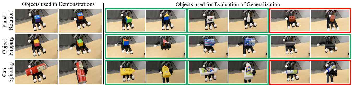
Fig. 5: On the left, we depict the start and end states of objects present in demonstration data. On the right, we depict the states produced by running our policies on objects not seen in demonstrations. Green boxes denote a successful rollout, while red boxes denote a failure.
