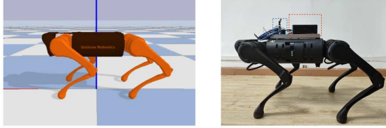
Fig. 4. Figure showing our quadruped robot Unitree A1 (right), and its simulation model in Pybullet [24] simulator (left). The UWB sensor and the onboard computer are circled by the blue and orange dotted lines, respectively.
