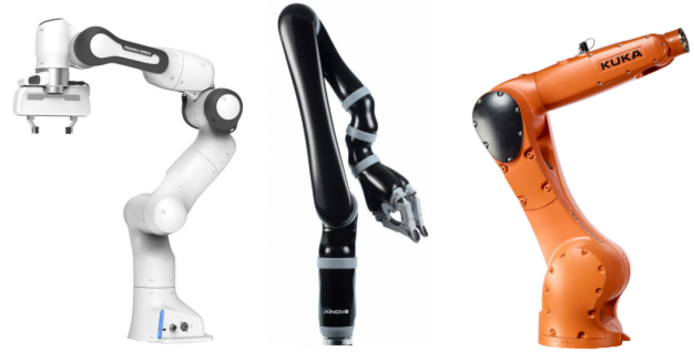
Fig. 1. Examples for robotic manipulators. left: Franka Emika Panda Cobot, middle: Kinova JACO 2 Cobot, right: KUKA KR 6 R900 sixx (KUKA AG)
