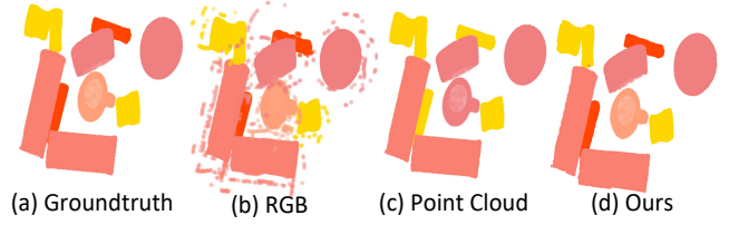
Fig. 5. The visualization of instance segmentation results for (a) groundtruth, (b) RGB-only (c) point cloud-only and (d) our methods, where partitions in different colors represent various classes.
