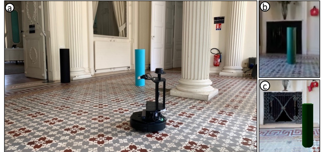
Fig. 1. We perform Multi-Object Navigation [41], i.e. the sequential visual search of multiple object in a given order, and are the first to do this in real physical environments (a) characterized by a large sim2real gap. This is illustrated by two first-person views (b), real and (c), simulation. We propose a hybrid method combining classical mapping and deep learning, and compare to the SOTA methods on this task using end-to-end RL training and auxiliary losses [28].
