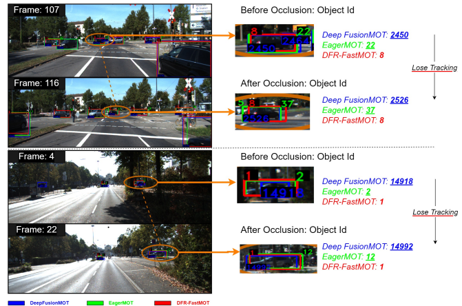
Fig. 1: Our approach recovered objects in two occlusion scenarios when DeepFusionMOT [4] and Eager-MOT [5] methods could not retrieve them.
