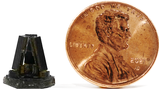
Fig. 1. Fabricated compliant microgripper using soft polymer actuator.
