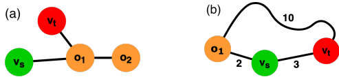
Fig. 3: (a) shows a simple connected graph where the objectives have to be visited twice to visit all destinations. (b) shows the case where revisiting the source v_s allows a shorter path when triangular inequality does not hold.
