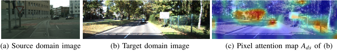
Fig. 3: Visualization of generated attention map A_{ds} . The difference between source domain image (a) and target domain image (b) is significant. That is, the source domain image has many city-style scenarios with crowded buildings, while the target domain image contains more countryside-style objects such as trees. Therefore, in this case, the attention map (c) of image (b) provides more attention clues (denoted in red in (c)) to extract target domain-specific features such as trees.
