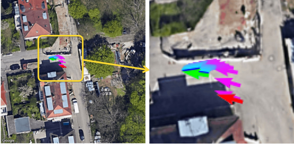
Fig. 4: The processing of pose optimization. RPRB optimizes the pose from an initial pose (red) towards the ground truth pose (green). The final estimation pose (blue). The color of the estimated pose during the process changes from red to blue.
