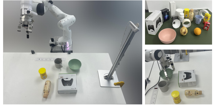
Fig. 6. A real-world experimental environment for object manipulation using a three-finger robotic hand and the given objects.
