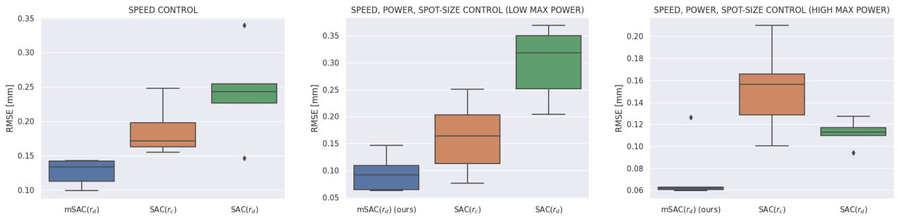
Fig. 6. RMSE comparison for the laser welding control task. Left: speed control. Middle: speed, power, and spot-size control (low max power). Right: speed, power, and spot-size control (high max power).
