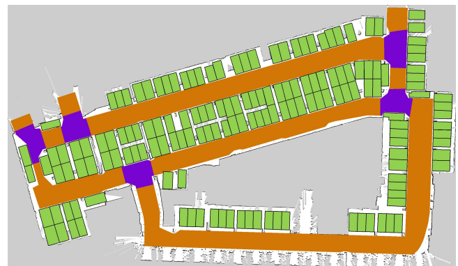
Fig. 2. The passable areas for a garage-cleaning robot with passages in chocolate, intersections in dark violet and parking areas in light green.
