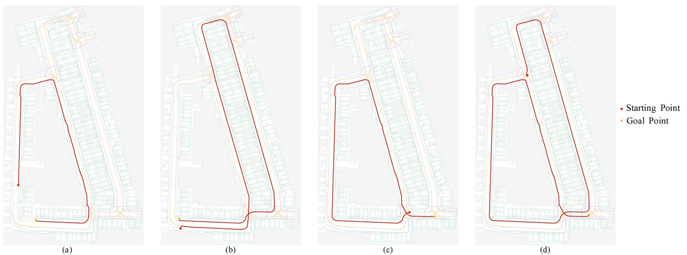
Fig. 1. Global path planning results when strictly complying with the road network that accounts for the traffic rules: (a) the starting and goal points are in the same lane and the latter is behind the former; (b) The starting and goal points are close but they are in the reverse lanes; (c) The starting and goal points are in different intersections and they are close to each other; (d) The starting and goal points are in different intersections and they are far away from each other.
