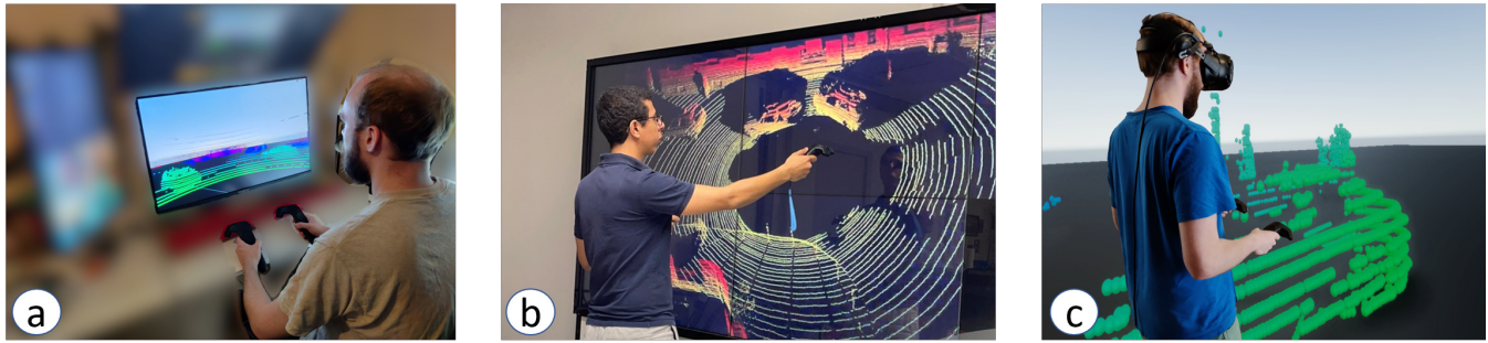
Fig. 2. Levels of immersion: (a) Non-immersive setup uses a 2D Monitor to interact with the scene. (b) Semi-immersive setup: the scene is visualized on a large 85" screen. (c) Fully-immersive setup: all 6 degrees of freedom are incorporated.
