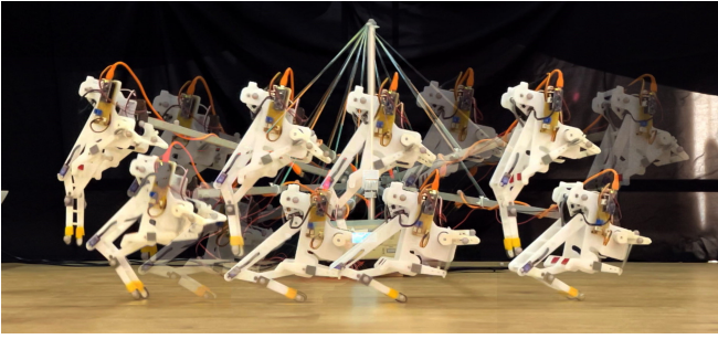
Fig. 5. Sequence of images for running and jumping in a place behaviors. Elastic bands are used to compensate connection rod's inertia
