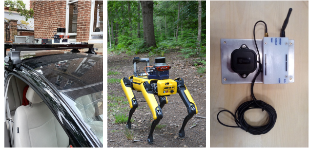
Fig. 1. Setups for experimental validation. Left: a car driving on public roads. Center: a quadruped robot moving in urban and forest environments. Right: a GNSS receiver carried handheld. Raw GNSS measurements were tightly fused with inertial sensing and optionally lidar using factor graphs.
