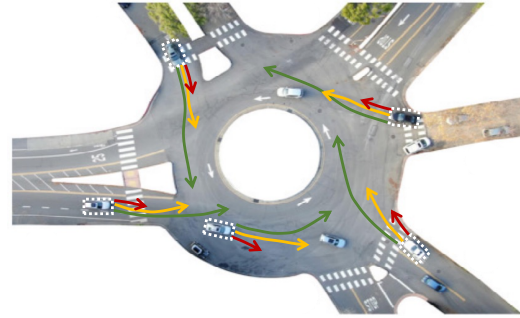
Fig. 1: With SHAIL, the ego vehicle learns to choose from a set of safe high-level options to navigate a complex driving environment derived from the Interaction dataset [7]. The learner requires only low-level expert states and actions as opposed to high-level actions or a reward function.
