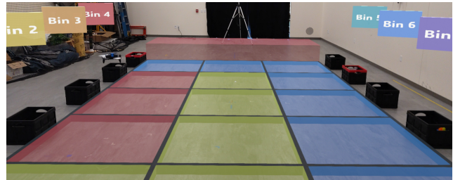
(a) View through the HoloLens from Home. Eight bins contain task components, a 3x5 grid indicates spatial ownership, and bin labels are selected to request access. Shown is a path to Bin 4.
