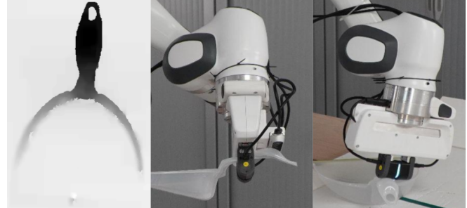
Fig. 1. Typical problem of planar grasps: the grasp center height is often set with an heuristic based on the highest surface. If the object's shape is unknown, this can lead to unsuccessful grasps. On the left, a depth grayscale image of an object generated from the point cloud captured by the RGBD camera mounted on the robot's end effector. On the center and on the right, two top-down grasps generated by Dex-Net [1] and GPD [10], two classical grasp generators. The Dex-Net grasp in the center is too low, the object is not grasped by the gripper jaws, while the GPD grasp on the right is too high to be successful. Without prior knowledge of the object and how thick it is, a wrong height prediction can lead to failure.
