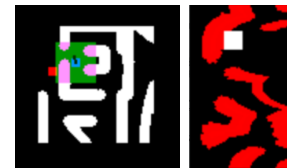
Fig. 2. Dummy training environment (left) with polar costmap (right).
