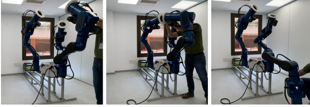
Fig. 12. A human operator freely manipulates the MARM arms under gravity compensation with joint impedance gains set to zero.
