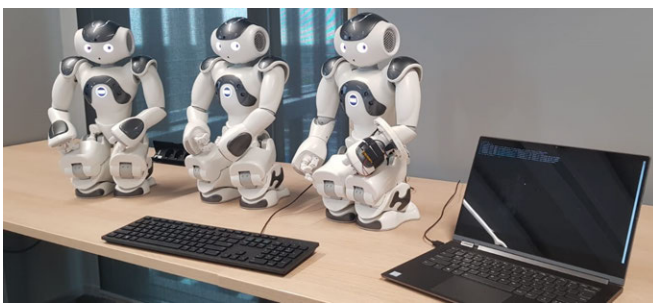
Fig. 5: User study setup. The left NAO is used to indicate the target pose in the Pose Mimic experiment, the middle NAO is used as baseline with the keyboard and the right NAO is mounted with KRIS.
