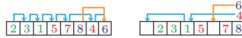
Fig. 4. Using a second buffer (indicated by the orange arrows), parallelism can be realized by arranging (574) and (86) in the same cycle group.
