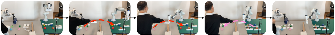
Fig. 9: Human-robot cooperative rearrangement. The arm needs to complete one local rearrangement by itself and one cooperative handover with the human.
