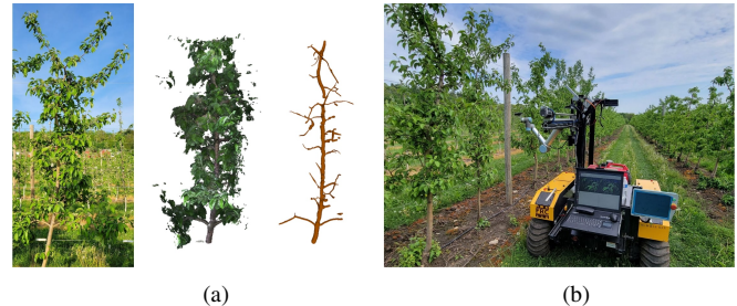
Fig. 1. (a) The 3D reconstruction (middle) and skeletonization (right) of a heavily occluded tree canopy (left). (b) Tree crops are tightly organized in rows in industrial orchard settings.
