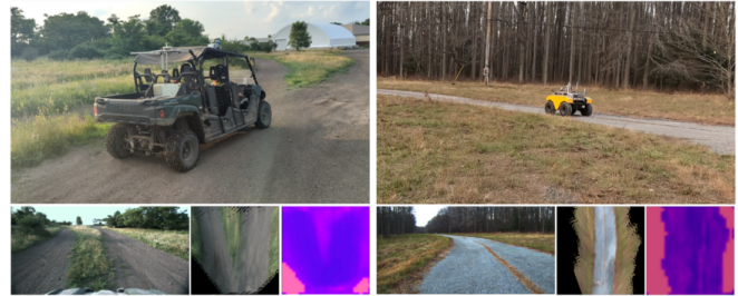
Fig. 1: We present a costmap learning method for off-road navigation. We demonstrate the efficacy of our method on a large ATV (left), and on a Warthog UGV robot (right).
