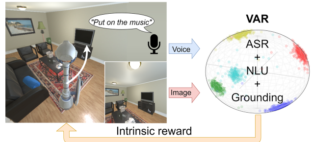
Fig. 1: Illustration of our method. The agent navigates and finishes household tasks according to a voice command. Windowed image shows the robot camera view. The voice and image received by the robot are the input to the VAR. The VAR is a unification of ASR, NLU, and grounding and produces an intrinsic reward that supports self-supervised RL training.
