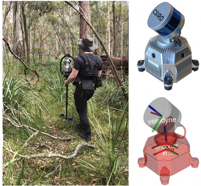
Fig. 2: Left: Image of sequence V-04 data collection campaign depicting the dense forest trails which are not accessible using vehicle or robotic platforms. Right: The sensor payload consists of a spinning lidar sensor mounted at an angle of 45^\circ to maximise field of view, a motor, encoder, an IMU, and four cameras.
