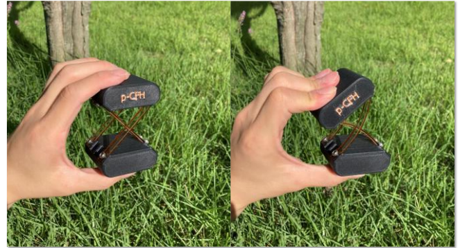
Fig. 1: paired-Crossed Flexural Hinge with rotating.
