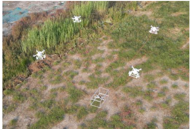
Figure 1. The multi-quadrotor transportation physical platform consists of four quadrotors. The payload is a rectangular aluminum frame connected to the quadrotors by cables.
