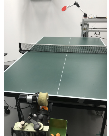
Fig. 1. Our setup consists of a four DoF robot arm actuated by pneumatic muscles and a ballgun that launches balls towards the robot arm. The robot successfully learns to return the ball to the desired landing point on the table. A color-based camera detection system measures the Cartesian positions of the ball.
