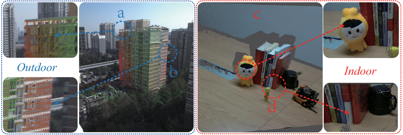
Fig. 11. Scene Left shows the result of point clouds reprojection in Livox MID-70. The color indicates the difference in depth. We can see that point clouds are clearly separated at the junction of the buildings in (a, b), which proves that the calibration result is reliable. Scene Right is the result of rendering the image into a point clouds in PyVista [32] captured by L515, the book spine and the doll is very clearly visible in (c, d).
