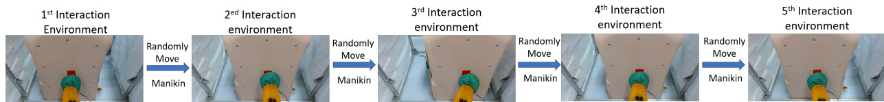
Fig. 5: Unknown changed interaction environments. The manikin was randomly moved such that both the interaction environment and the tracking target (i.e. the red label on the manikin’s back) were changed. The soft robotic manipulator was controlled to be adaptive to the changing environment and track the target.
