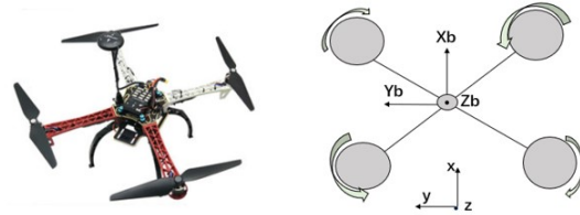
Fig. 1. A UAV in the X configuration with four motors and four rotors. The direction of motor rotation and the axis are shown in the picture.
