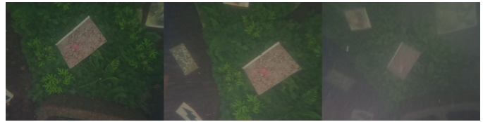
Fig. 6. Image samples in EASI dataset of three turbidity levels. From left to right: Clear, Medium, Heavy.
